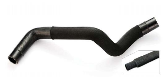
FT-HSS heatshrinkable textile sleeve consists of polyester multifilament and special modified polyolefin monofilament, the shrink ratio is 2:1, the special woven construction makes it very flexible, it can be easily cover on the hoses with irregular shapes. It is suitable for used in rough environments, providing excellent abrasion resistance and noise reduction.
